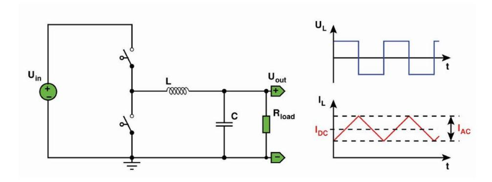
By post-processing of the transient inductor and current waveforms, the inductance, the AC and DC power loss and dynamic saturation can be calculated [3]:
